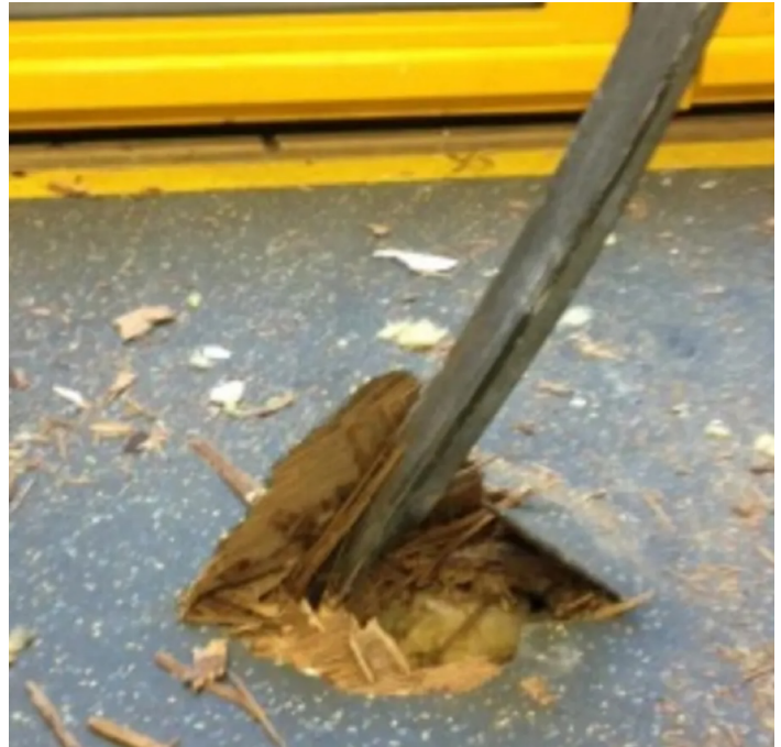
Rail that penetrated the bottom of a coach
